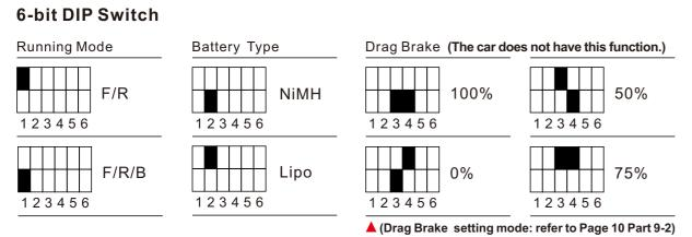
The ESC parameters can be set by the 6-bit DIP Switch of the transmitter, that is, the DIP switch is located at different positions and the corresponding parameter values are different. There are three parameters can be set for the ESC, which are "Running Mode", "Battery Type" and "Drag Brake".
